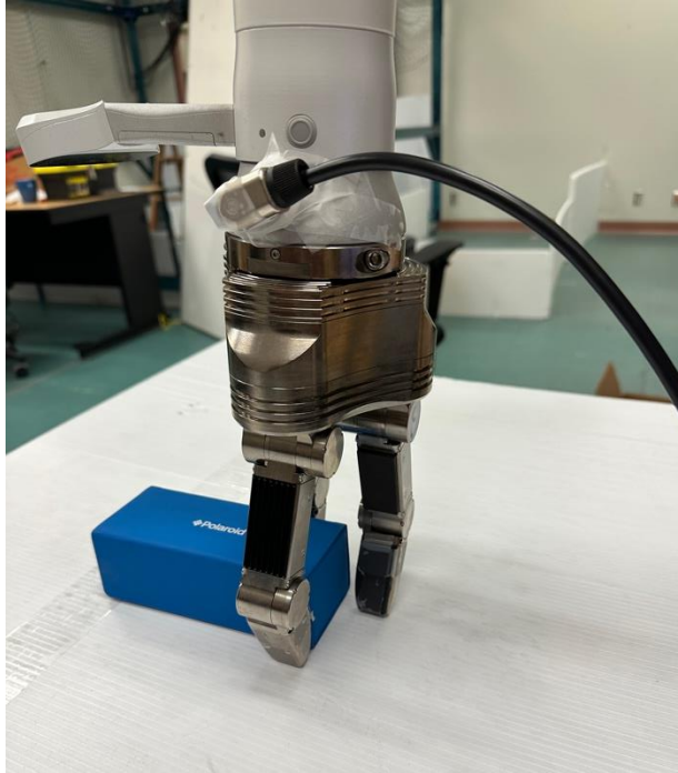
Figure 4.2: Unsuccessful grasp because one finger missed the object while it was closing.
