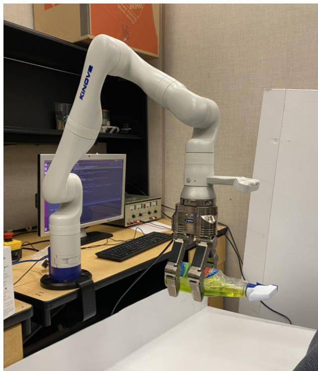
Figure 2.2: Schunk SDH robotic hand attached to the Kinova kortex Robot gen3 robotic arm. The robot is in the view from the top grasping configuration.
