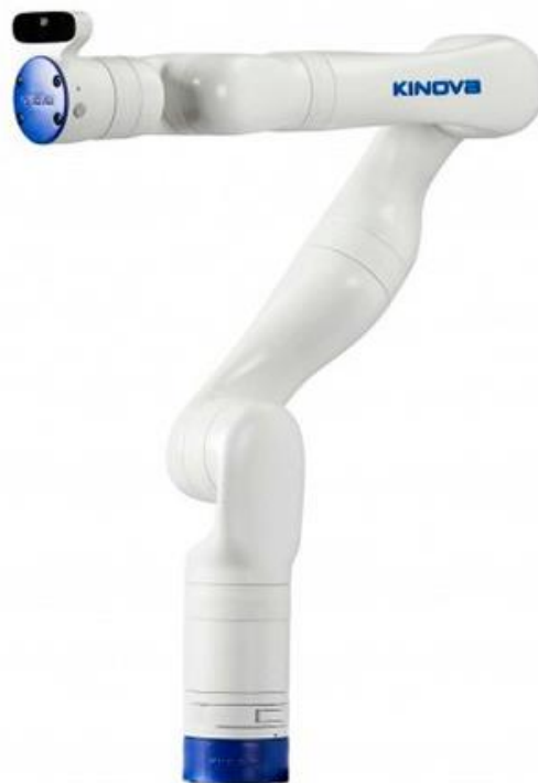
Figure 2.5: Kinova gen3 robotic arm with 7 degrees of freedom.
