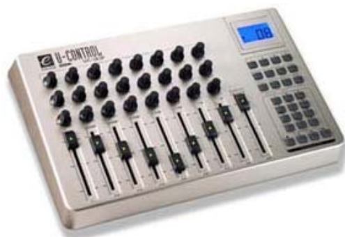
Figure 5 Controller device with rotational dial (top) and vertical slider (bottom) (see online version for colours)
