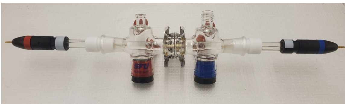
Figure 11. The H-cell used in this work was made by the Simon Fraser University glass blowing shop. A metal clamp and O-ring seal a membrane inbetween the two compartments. Openings in the top allow for CO 2 to be bubbled in. Ag/AgCl reference electrodes are shown, as sourced from Pine Analytical.
