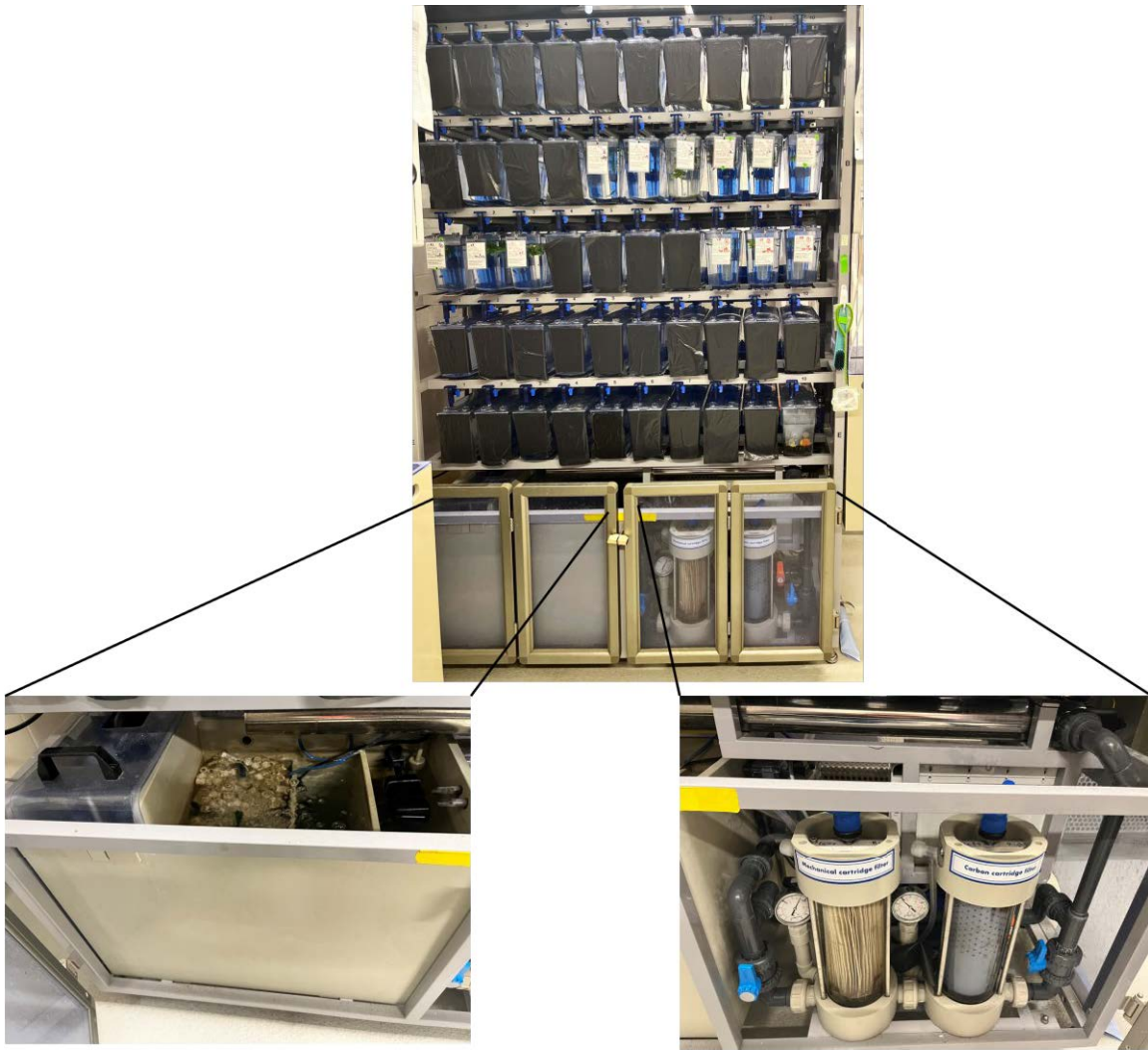
Figure 11: A photograph of the ZebTec zebrafish rack system, with magnified portions showing the filtration systems.
