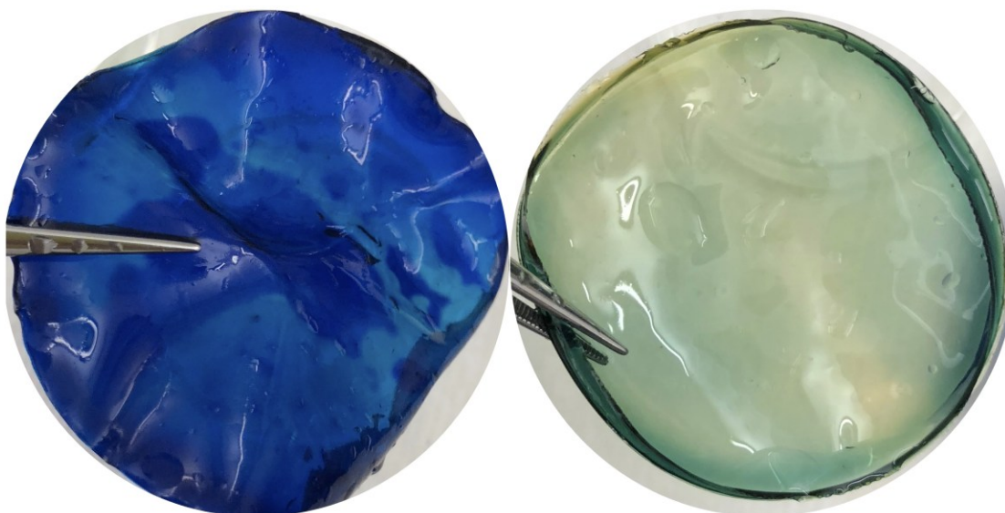
Figure 4-7. Color change of the thymolphthalein and HMT-PMBI co-casted membranes. The membranes were initially exchanged to its OH - form by immersing in 1 M KOH. A lighter blue band was observed after adding a small chunk of dry ice for the membrane co-casted with an indicator to polymer ratio of 1:10 2 (left), while a yellow band was observed for the membrane co-casted with a 1:10 3 indicator to polymer ratio (right).
