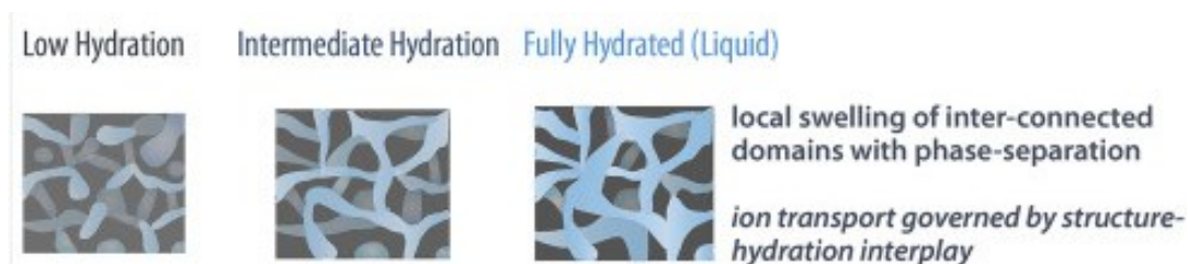
Figure 1-6. Schematic of anion exchange membrane at various hydration level. Adapted from ref 31
