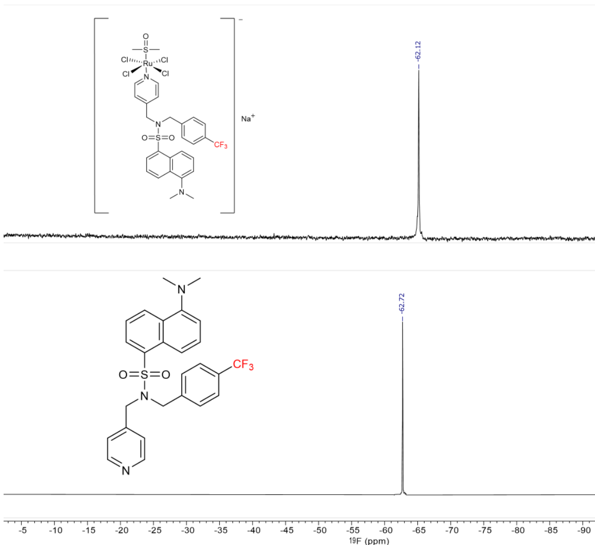
Figure 2.5. Upfield shift of the fluorine signal upon attachment of 2-4 to Ru(III).
