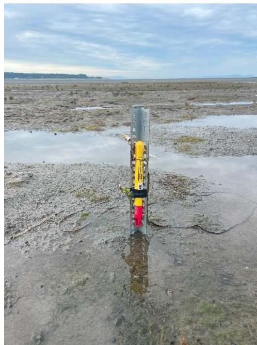
Figure 5: Image showing an RBRsolo instrument attached to a perforated L-shaped angle bar at the S1 LDPP study site in Boundary Bay, British Columbia, used to obtain wave data from October 2023 to January 2024.
