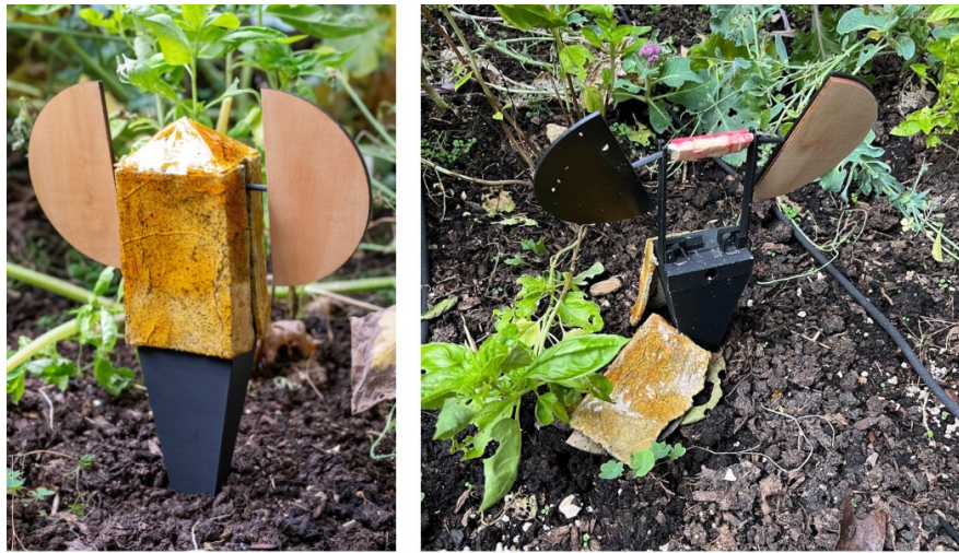
Figure 21. wi-fi-notifier enclosure with the paddle placed in garden (left); Damaged remains of wi-fi-notifier after about a month (right).
