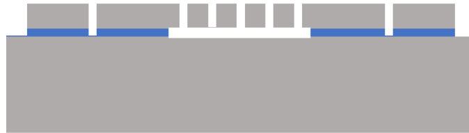
Figure 5-21 Schematic cross section of the devices after release
