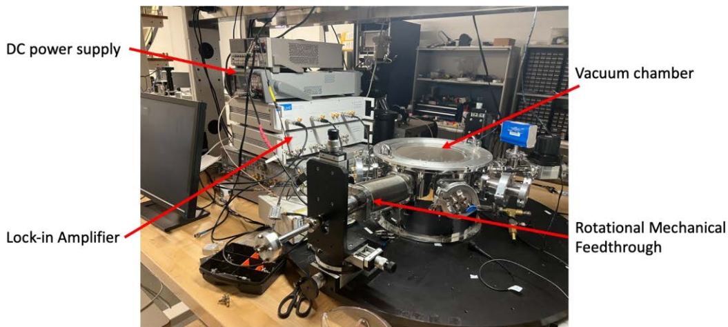
Figure 6-6 Schematic of the measurement setup for characterization of resonant accelerometers
