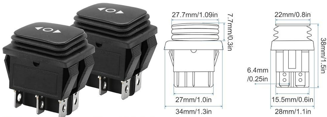
Figure 14: (a)Switch Image - (b) Switch Dimensions [30]
