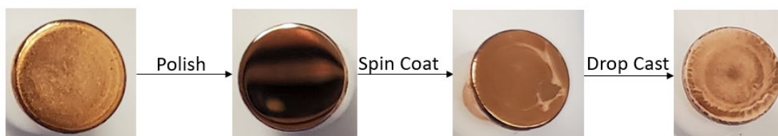
Figure 1. Images depicting select steps in the process of preparing a polished copper (Cu) stub followed by spin coating and ultraviolet (UV) irradiation to create a thin film of cross-linked SU-8 polymer onto which zeolite particles are then deposited through drop casting.
