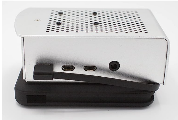
Figure 3.1.8.1 - VGE Battery pack attached to an encased raspberry Pi Controller
