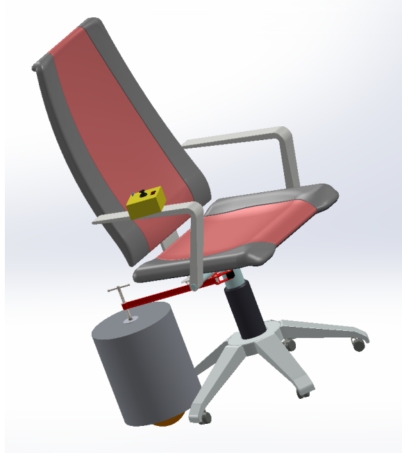
Figure 2: Overview of Chairable with controller attached to a office chair [1][2][3][4]
