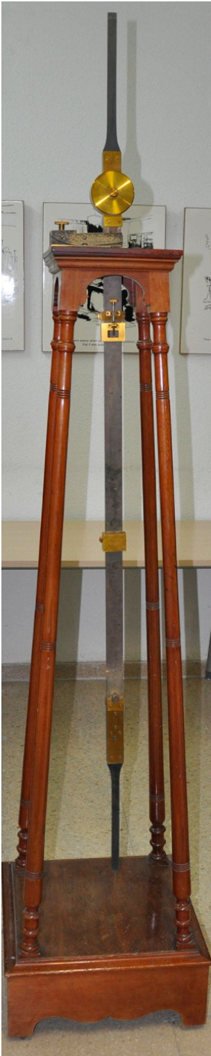
Figure 2.6: Kater Compound Pendulum (Wikipedia contributors 2023b)
