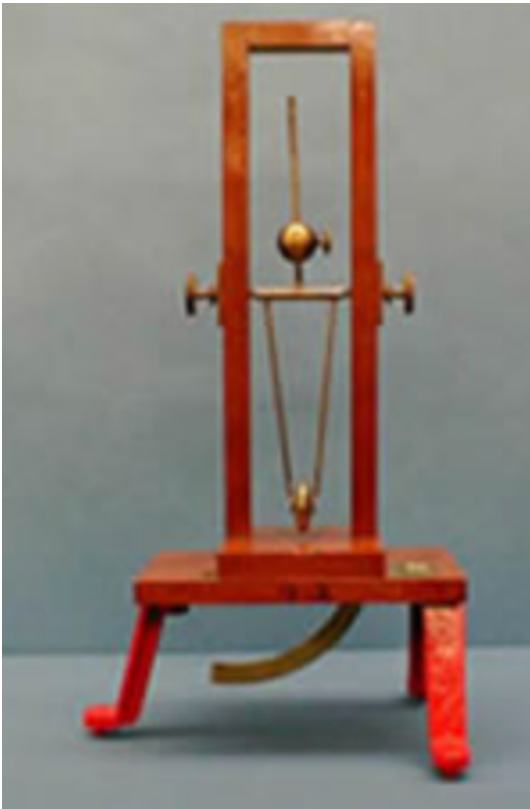
Figure 2.4: Compound Pendulum (Purdue Physics and Astronomy 2023)
