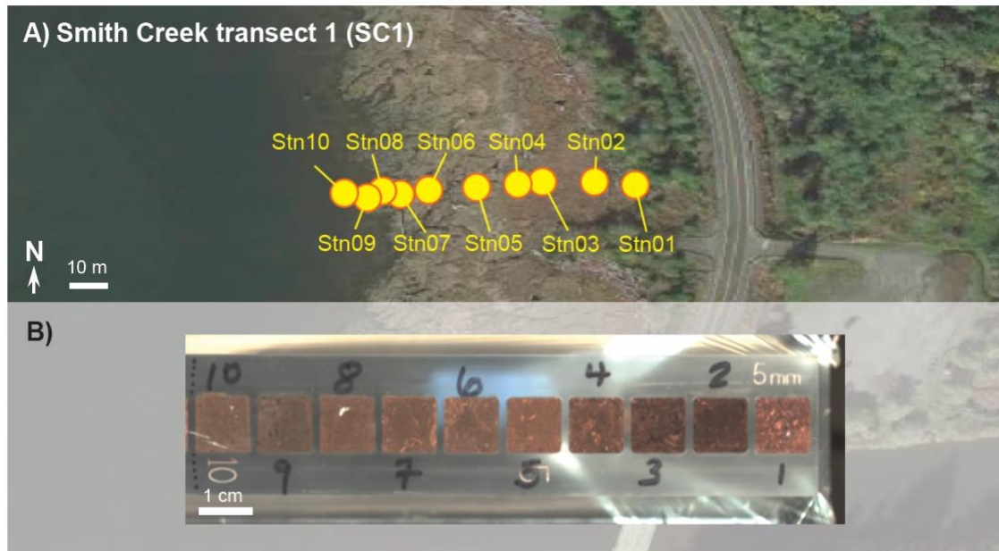
Figure 3-3 Example of surface sediment in sequential sample reservoirs (SSR) (A) Smith Creek transect 1 (SC1) with station labelled. (B) SC1 surface samples prepared and loaded into SSR for XRF analysis on the ITRAX-CS.
