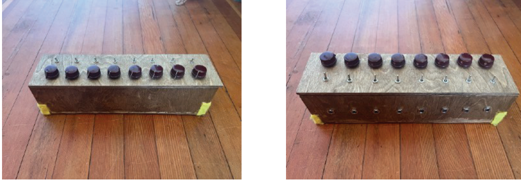
Figure 8. controller for the motors (completed)
