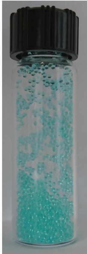
Fig. 34: Collected microcapsules (contain liquid desiccant: 60 wt% LiBr and 40 wt% deionized water).
