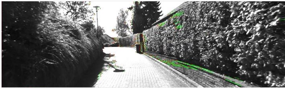
Figure 4.4: Example Keypoint Placement with Semantic Segmentation Boundaries.
