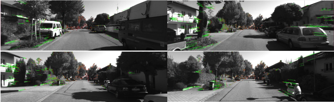
Figure 4.8: Inconsistencies in Keypoint Placement for the Same Object Between Frames
