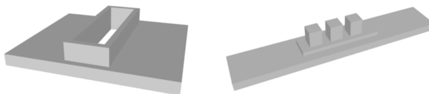
Figure 3. Drawings of PDMS device mold: side piece (left) and bottom piece (right).
