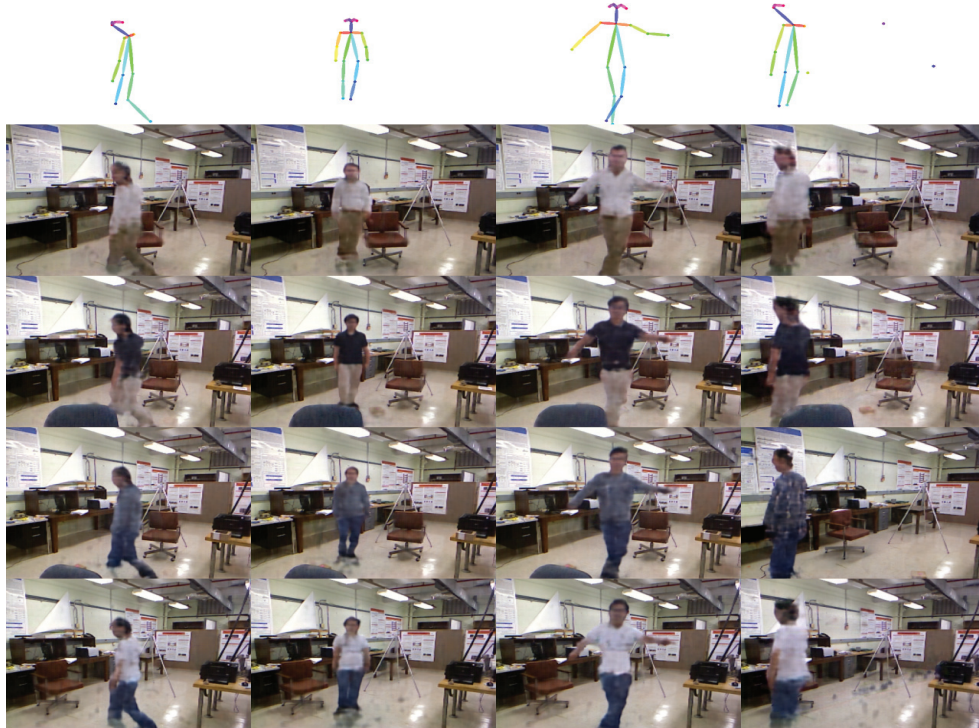
Figure 4.6: The screen shot of a video generated by UTK expansion. The first row shows skeleton clips extracted from an arbitrary action. Second to fourth rows show the generated video for subjects from different clip carrying out that specific action.
