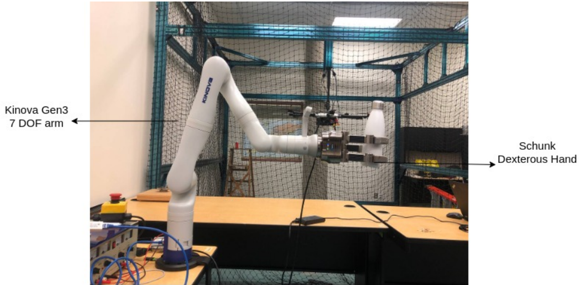
Figure 1.3: Kinova gen3 robotic arm and Schunk Dexterous gripper in handover configuration.
