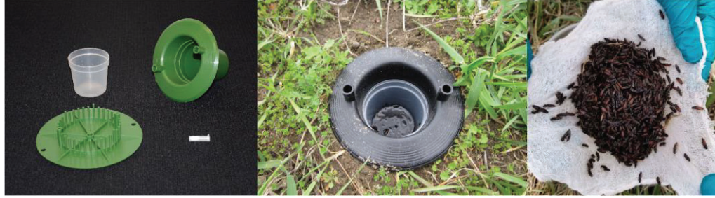
Figure 2.2. (A, B) Photographic illustrations of a Vernon Pitfall Trap ® [(A) trap parts: 1-trap bottom, 2-trap lid, 3-180 ml insert cup, 4-pheromone receptacle; (B) a trap bottom installed in the field for testing limoniic acid or its analog in field experiments; and (C) a representative example of Limonius californicus males captured in a single trap over the course of one week during the beetles' peak swarming period in Granum, Alberta. Photo credit (B): David Shack
