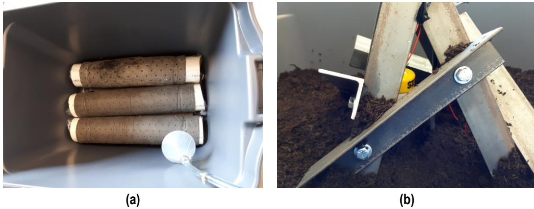
Figure 22: (a) Plastic pipes at the base of the tote for self-watering and; (b) electrode placement in the tote
