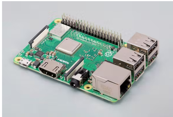
Figure 17. Image of Raspberry Pi 3 B+ [9].
