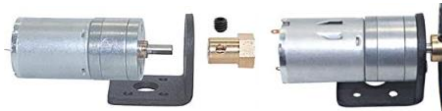
Figure 9. DC motor fixed to a motor mount [7]
