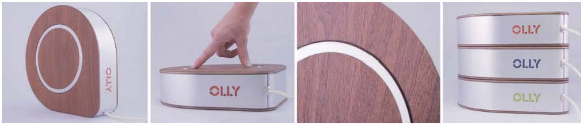
Figure 33: Left to Right. Olly can operate standing up (or lying flat); A pending song is played by gently spinning the rotating disc (pictured here when lying flat); Woodgrains move in and out of alignment as the disc rotates; Three Olly design artifacts.
