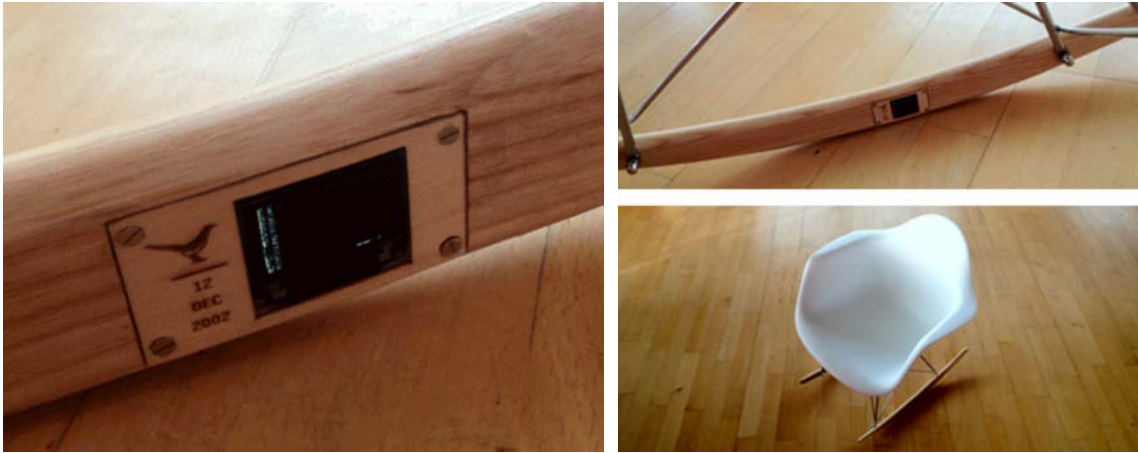
Figure 6: Long Living Chair is a rocking chair with enhanced memory, which knows the day it was produced and can record how many times is used over the course of 96 years. Images retrieved from Pschetz and Banks' paper in 2013 [180]
