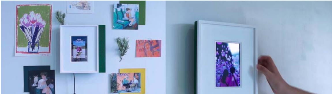
Figure 5: Slide2Remember installed on the wall of the home, showing the user's photo and playing music that the user heard in the same period during which the photo was taken Images retrieved from Kim et al.'s paper in 2022 [114]
