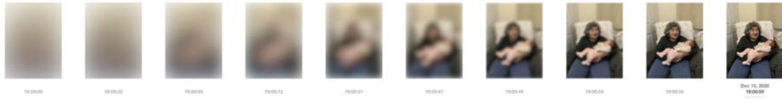
Figure 28: An example of how the PhotoClock system deals with empty moments. It applies Gaussian Blur to the picture every second at a level based on how far the picture should appear in time.
