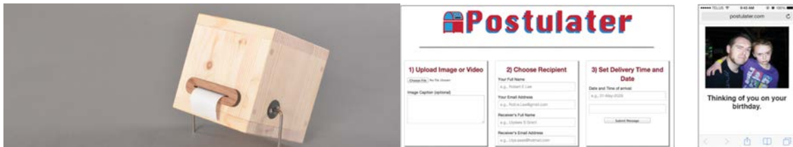
Figure 7: Reflexive Printer prints a halftone photo from its user's smartphone on thermal paper, and deletes it; Postulator is an online application that allows users to send multimedia messages, including images or videos, to a future date and time. Images retrieved from Tsai et al.'s paper in 2014 [223] and Hawkins et al.'s paper in 2015 [87]
