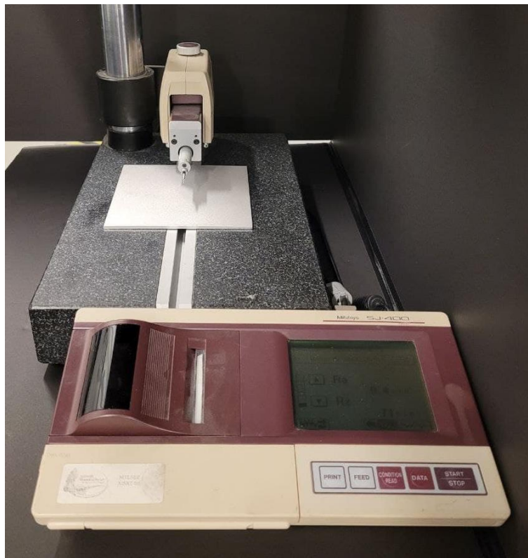
Figure 13. A Mitutoyo SJ-400 surface roughness tester
