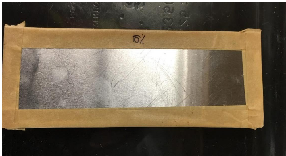
Figure 16. Taping of the substrate to maintain 0.2 mm thickness for coating
