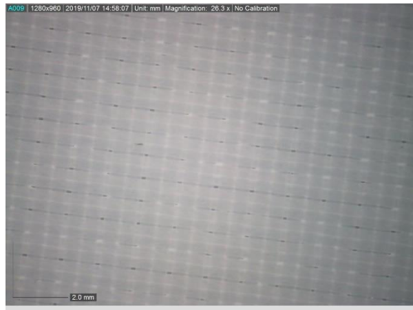
Figure 29. A microscopic view of the 3D printed test section coated with epoxy (XTC-3D™ [115])
