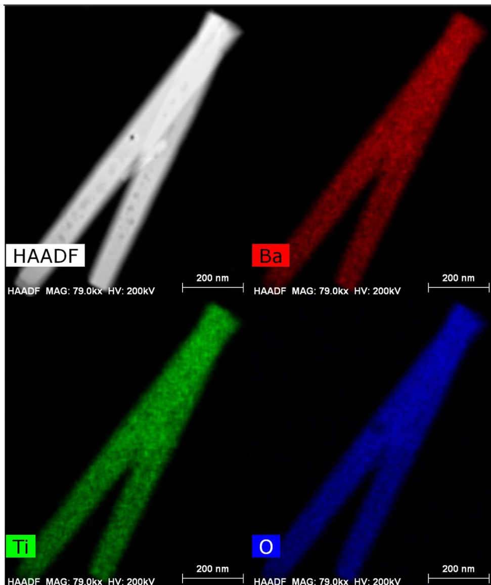
Figure 5.4. HAADF image (top left) and a series of EDS spectra of a BaTiO 3 particle that was synthesized in 9:1 (v/v) ethylene glycol:diH 2 O at 180 °C using SDS as the surfactant.
