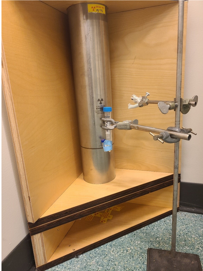
Figure A1. General setup of irradiation experiments in front of the neutron generator for both \text{BaTiO}_3 and S samples.
