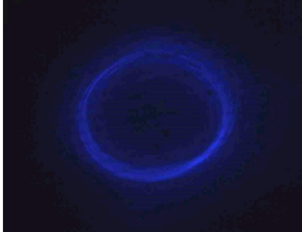
Figure 8.37. Front view of cantilever scan for vibration at its resonant frequency.
