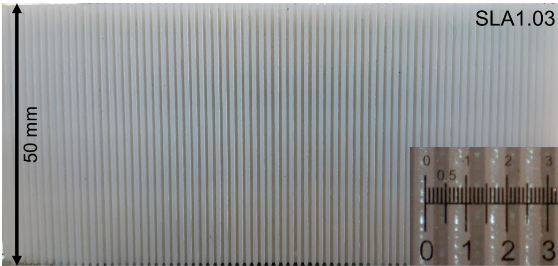
Figure 30. Micro-grooves made by stereolithography (SLA1.03) were used for the capillary rise measurement. The inset shows a micro-groove thickness of 500 \mu\text{m} and a micro-groove width of 400 \mu\text{m} . Micro-groove depth is 1 \text{ mm} . Table 4 lists the sample details.
