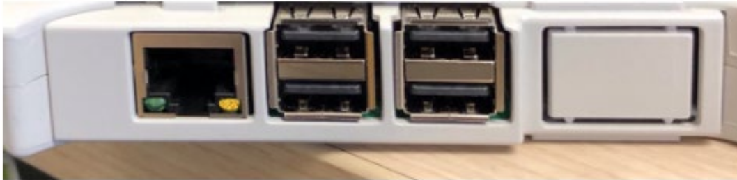
Active State: Capture Tool is on and connected to network system
