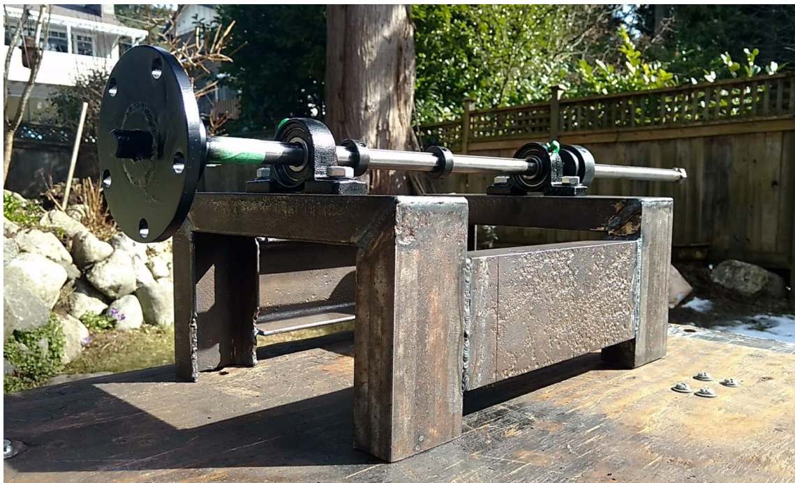
Figure 3.6: Rotor Adapter and Hub Installed on Shaft and Painted (Front View)
