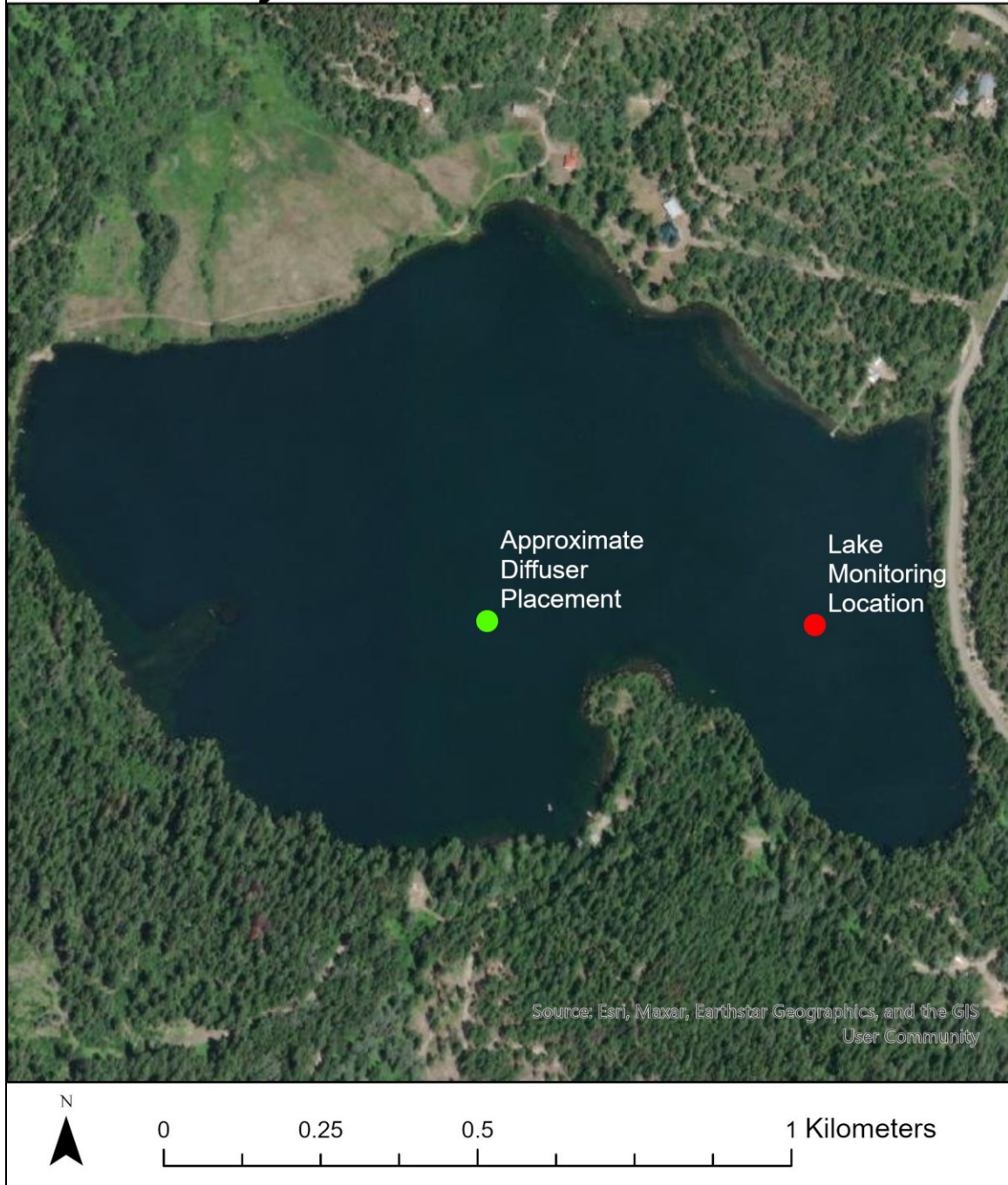
Figure 18. Approximate location of the aeration diffuser and the monitoring station to be used while destratification is in progress.
