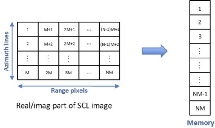
Fig. 3.6. Storing the SLC image in hardware
