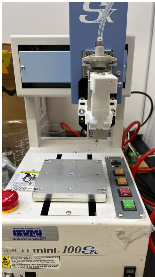
Figure 3.2. Overview of the Musashi printer for DIW printing.
