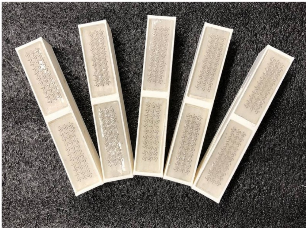
Figure 3.4. Five electrodes for the detection of EMG from five fingers.
