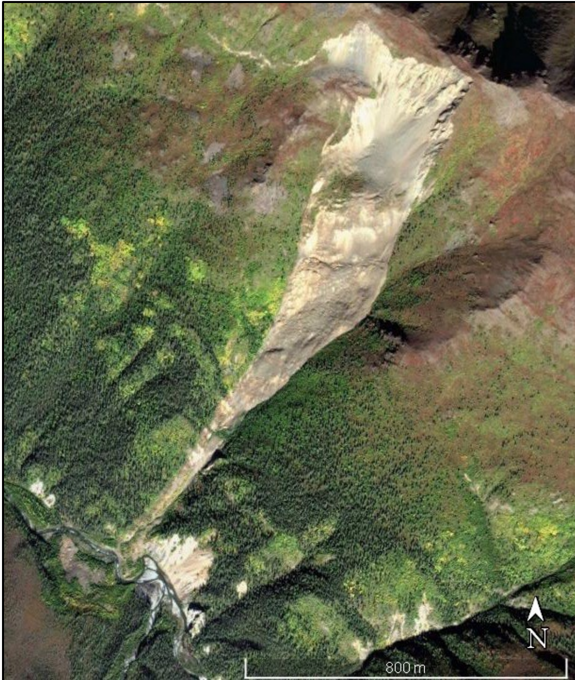
Figure 3.12. Generic rock slide as it appeared in 2010. Landslide morphology appears similar to what was observed during the 2019 field season. Exposed bedrock is observed in the feeder gully as it enters the valley bottom. The modern river now bisects the toe of the deposit. Alders were growing on the deposit and were surrounded by conifers on the perimeter; this helped delineate the extent of the landslide. A distinct change in vegetation type from younger deciduous growth on the deposit to more mature conifer growth around the landslide was evident in air photos as well as in the field. Image courtesy of Google Earth.
