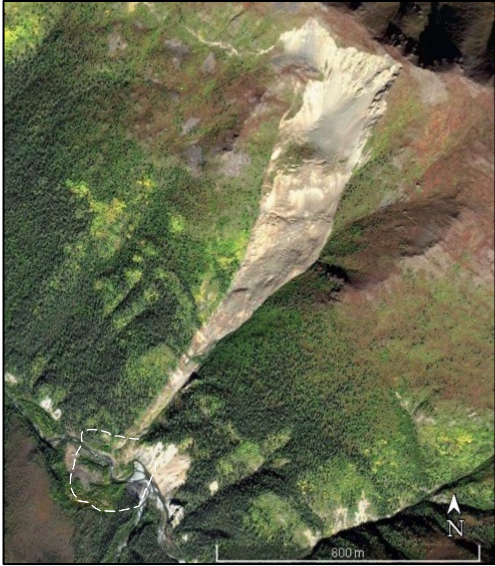
Figure 1.24. Generic Landslide. The debris in the valley bottom is outlined by the white dashed line. The head scarp and trace of propagation are clearly visible and distinguished by the lighter brown tone. ©GoogleEarth, 2019.
