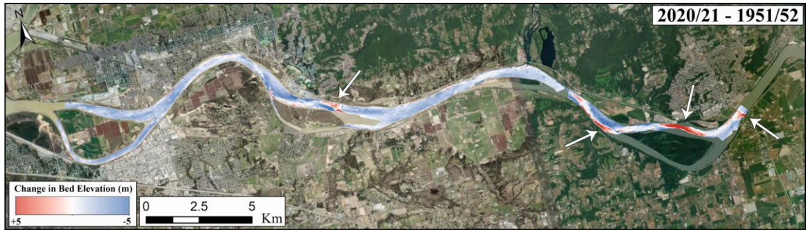
Figure 2-7. Bed elevation difference map of the 2020/2021 and 1952 bed surface. The white areas highlight locations where negligible bed change occurred, while blue represents relative lowering and red represents relative deposition between the two surveys. Arrows indicate notable locations of bed aggradation.
