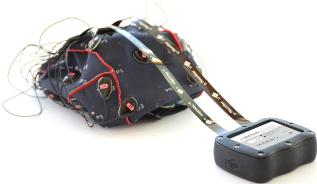
Figure 2.4 EEG dry electrode cap. g.tec medical engineering, GmbH. Brain-Computer Interfaces & Neurotechnology ( www.gtec.at ).
