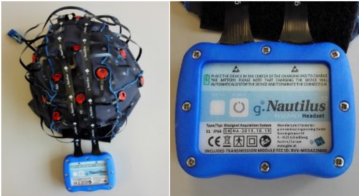
Figure 2.3 EEG gel-based electrode cap and acquisition device. g.tec medical engineering, GmbH. Brain-Computer Interfaces & Neurotechnology ( www.gtec.at ).
