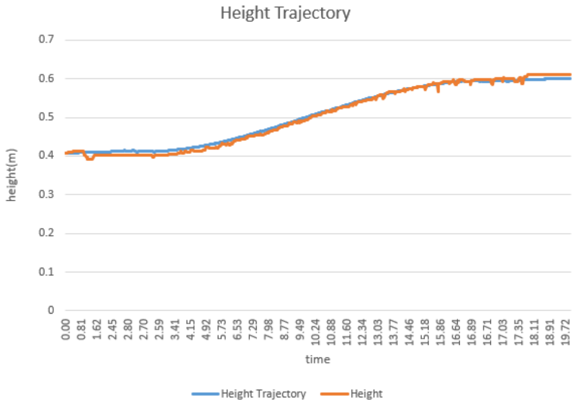
Figure 6.12: Trajectory tracker using cascaded PD controller and motor current controller (Height Response)
