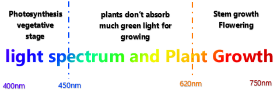
Figure 1.1: Light spectrum output of a LED as a light source and light-wave used by plants during different growing stage
