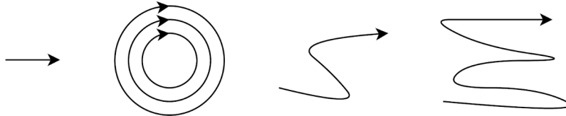
Figure 3.7: Visualization of person motion model. From left to right: moving straight, in different circles, in smoothed curves and using annotated simulated path of a human.
