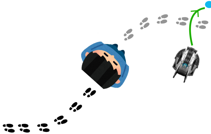
Figure 3.4: A mobile robot following-ahead of a user. The robot must predict the user’s trajectory to stay in the correct relative position. In each time step in our proposed approach, the robot considers previous states of the joint system to generate a goal (blue dot). Then a trajectory planner navigates the robot towards the goal (green line).
