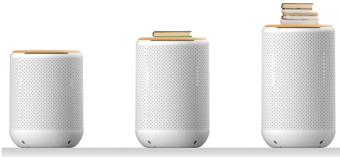
Figure 5.2. The deformTable is a shape-changing artifact upholstered with a piece of elastic fabric (rendered image). From left to right: deformTable in a static state; a book is placed on the table surface of deformTable; deformTable goes up higher as more books are placed on the table surface.
