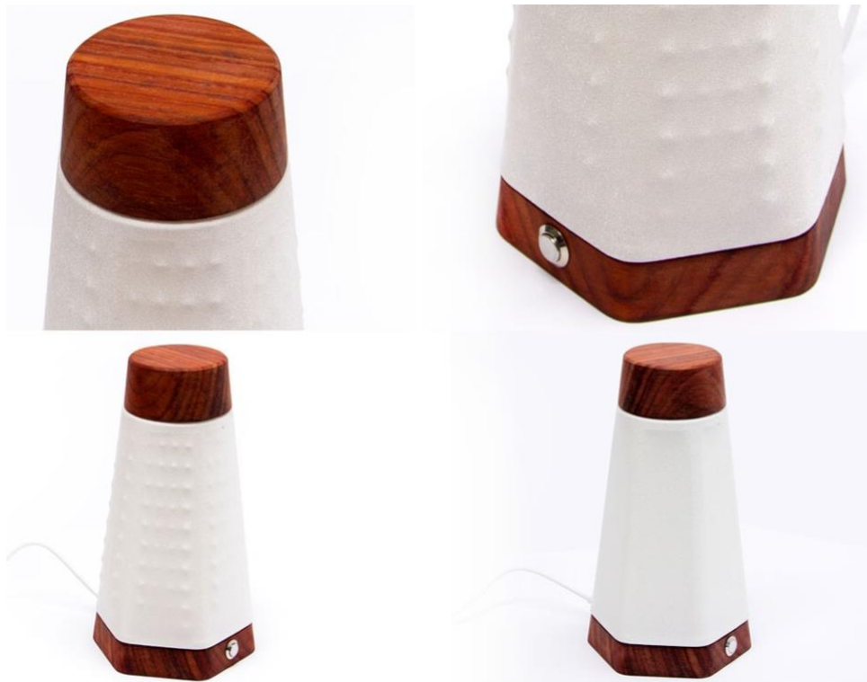
Figure 4.2. Clockwise from top-left: a power switch installed at the base of transTexture; a rotary button that can control both the digital light and lampshade deformation simultaneously; the fabric lampshade in a shape-changing state; and a static state.
