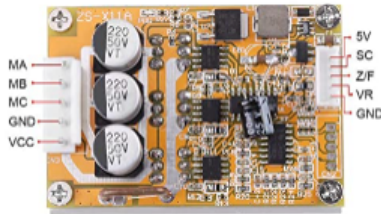
Figure 13: Brushless Hall Motor Controller Speed Controller 5V-36V 350W
