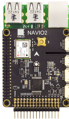
Figure 5.1.2 - Raspberry Pi with Navio2 attached to the pins
