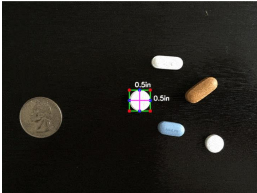
Figure 4.3.1: Measuring the size of the object using OpenCV[4]
