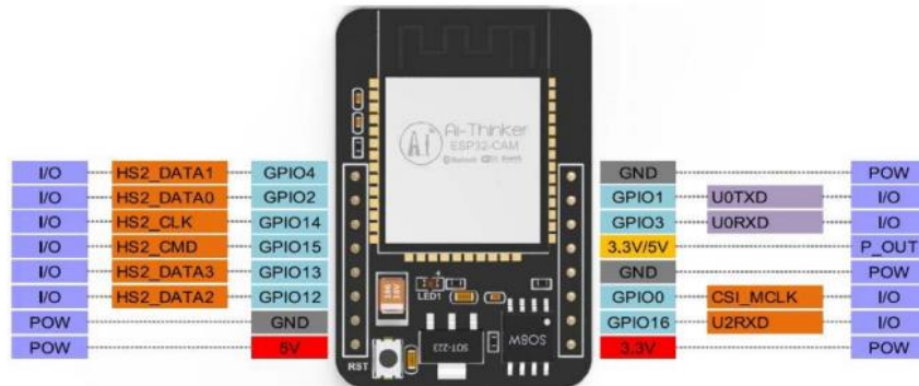
Figure 3.1.2 ESP32 Cam Module Pinout[1]
