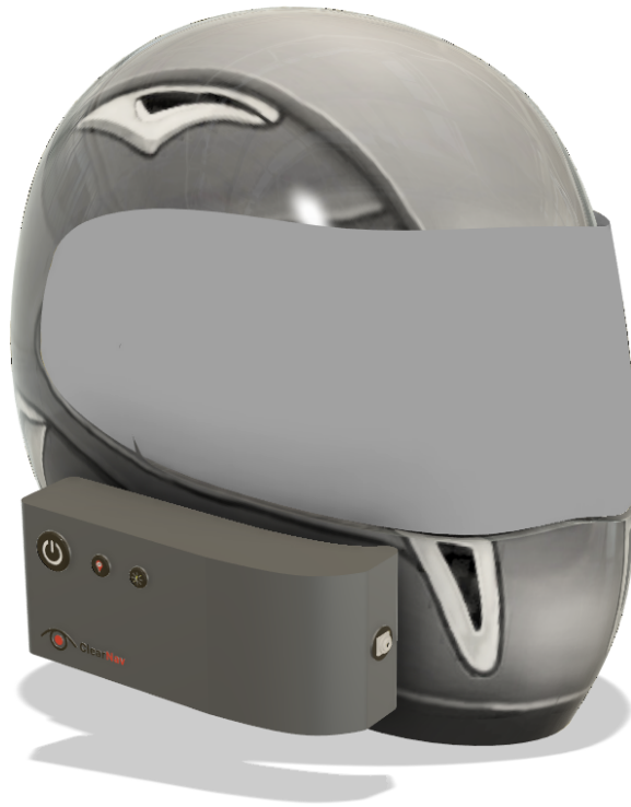
Figure 3.2.1 - EZhud Mounted on Helmet (Helmet From [9])
