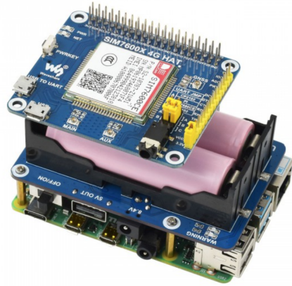
Figure 9: UPS hat with 18650 Li battery [7].
