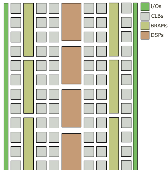
Figure 2.1: FPGAs consists of IOs, CLBs, BRAMs and DSPs
