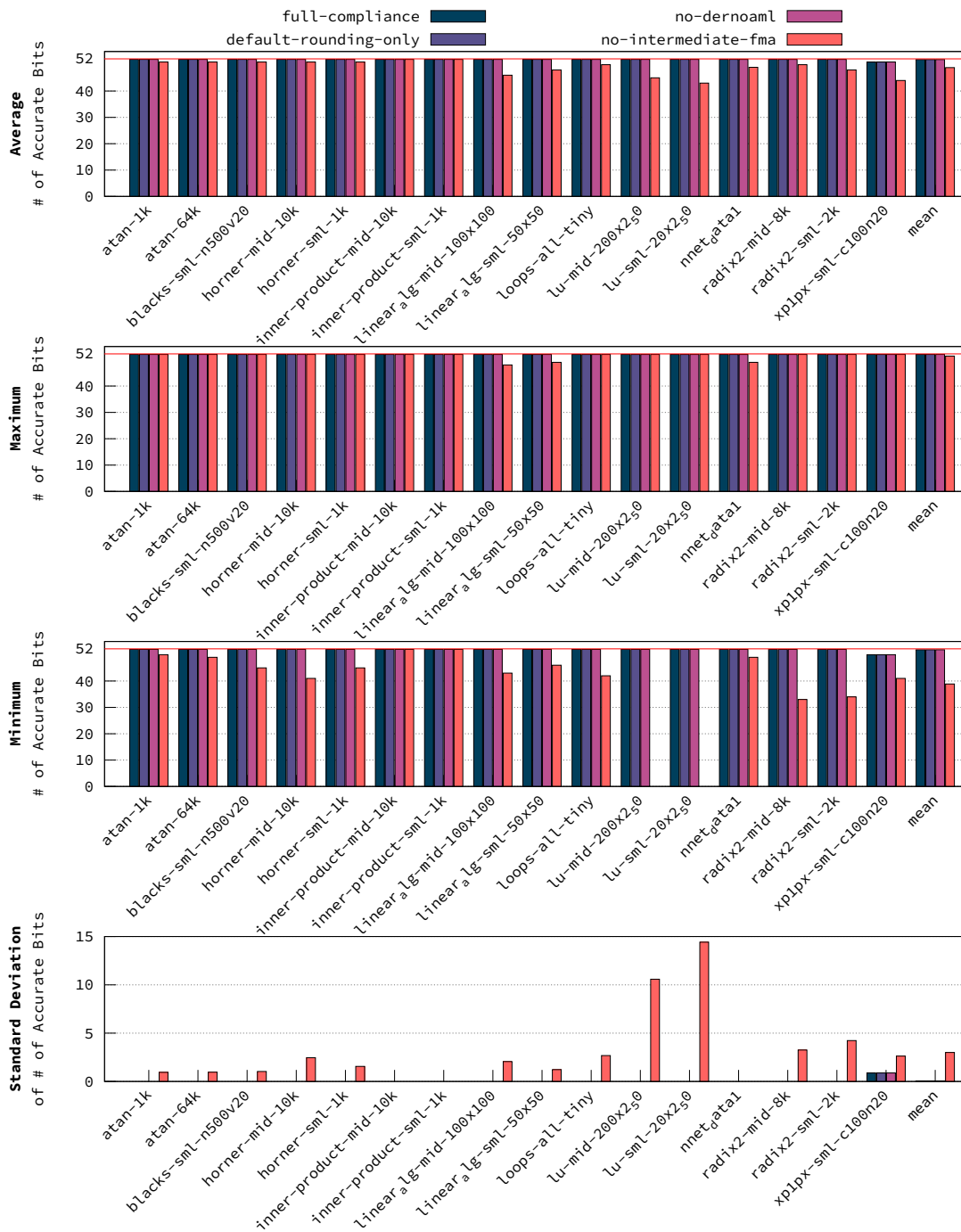
Figure 5.1: The FPMark’s self-verification passes when average, maximum, and minimum number of accurate bits are 52 (DP).
