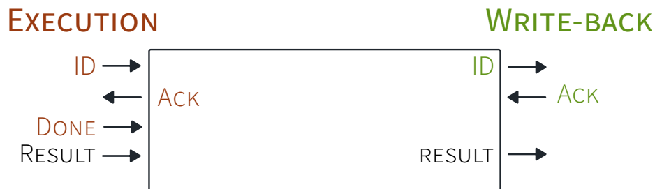
Figure 3.11: Interface connecting the execution units and the write-back stage.
