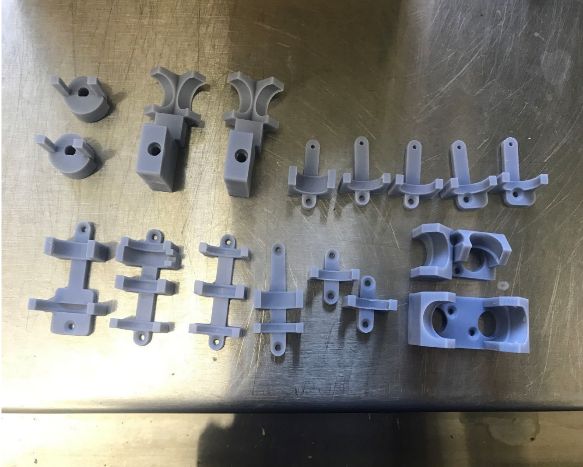
Figure 3.12. Picture of optical mounts used in OPA. All mounts were printed using a stereolithography (SLA) 3D printer (property of the author of this thesis). ELEGOO ABS-Like photopolymer resin was used (sourced from Amazon.ca). The printing process is depicted and described in Figure 3.13.
