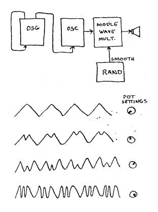
BOTTOM WAVE MULTIPLIER: Like the Middle Multiplier, the Bottom one also has two independent (but identical) inputs. Both inputs are AC coupled. The general effect of the module is that of a full-wave rectifier for audio signals, which means that negative voltages are "flipped" up into the positive.
