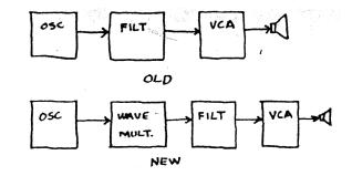
UPPER WAVE MULTIPLIER: The Upper module of the trio is a the simplest of the three. It has a switch for two different settings characteristics. In the HI setting it acts to moderately "square up" or soft clip the signal. The soft clipping is amplitude dependent, producing changes in timbre as the loudness increases.
