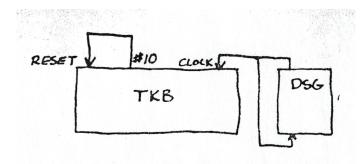
In this patch, just like in the previous one, the sequence will return to stage #1 only if that was the last keypad touched, otherwise, it will reset to whatever pad was last touched. In the above patch you can get the sequence to activate stages 5,6,7,8,9 and then reset to 5 by tapping stage 5's keypad. By tapping different keypads different length sequences can be "plated", each ending at stage 9.
