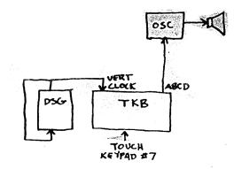
If in the aboe patch, stage #7 is now activated by touching its associated keypad, the four pots in stage #7 will determine ABCD's output.
