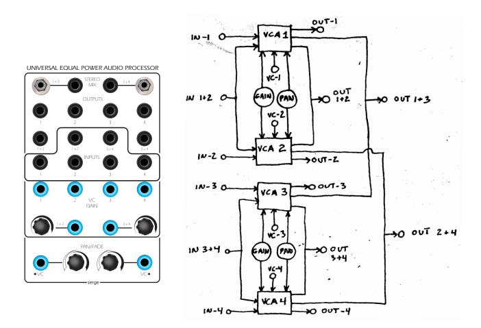
Each VCA can be used seperately with signal input at 1,2,3 and 4 respectively. A signal to input 1 + 2 will be sent to VCAs 1 AND 2 for panning and an input to 3 + 4 will be sent to VCAs 3 AND 4. These "dual" inputs can be mixed with the individual inputs to the VCAs.
