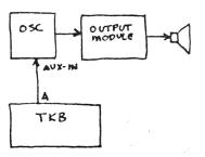
In the above patch the processing pot associated with the AUX-IN processes the incoming voltage from the TKB. Below are some typical processed TKB voltages:
