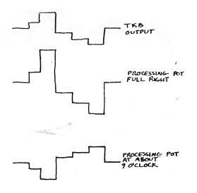
5.6 It is convenient to think of the TKB in this manner: All the pots in each row are tied to a common output (output A for the pots in row A for instance) but only one pot is activated and that is determined by which keypad was last touched. Since there are four rows, four parameters or modules can be controlled in 16 pre-set ways and these pre-sets, or stages, can be accessed directly by the touch pads.
