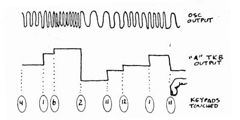
Patched in this fashion, none of the pots in Rows B, C, or D have any effect. However, if it is re-patched so that the output of the TKB is taken from the B output instead of the A output then only the pots in Row B will Be active. The same is true for Rows C and D. It is possible to use all four of these outputs (or as many as needed ) SIMULTANEOUSLY as in the Patch below.
