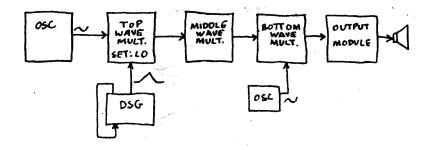
DUAL UNIVERSAL SLOPE GENERATOR (DSG). The DSG can function as a non-linear lo-pass filter essentially by softening the slopes of the IN signal. Generally speaking, the less steppingstones the slope of a waveform the fewer high frequencies it contains. To accomplish this the RISE and FALL times must be set quite fast. Increasing either the Rise or Fall time will increase the filtering action.
