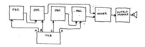
Now at each stage the pot in Row A controls the frequency of the Modulating OSC while the pot in Row B controls The base frequency of the modulated OSC. Row A and B could be replaced by any two rows. By touching the Sixteen different keypads and setting the appropriate pots, sixteen different sounds can be set up and recalled In any order at the touch of a finger.
