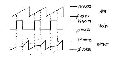
3. LOW FREQUENCY OSCILLATOR: [CYCLE] ---> [IN] APPEARING AT SMOOTH OUT IS A TRIANGLE WAVE WHOSE FREQUENCY IS CONTROLLED BY THE [RATE] OR VC INPUT. IN THIS INSTANCE [CYCLE] IS A PULSE TRAIN (WAVE) OF THE SAME FREQUENCY AS THE TRIANGLE WAVE. [HOLD] STILL FUNCTIONS AS WELL.
