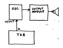
The TKB has four rows of pots across, labelled A,B,C, and D, and one row of keypads. There are 16 columns each with four pots (ofe from each row) and one keypad. At any given instant ONE and ONLY ONE column is activated and this is indicated by an LED (Light Emitting Diode) on the keypad of the respective column. These columns will be referred to from now on as STAGES.
