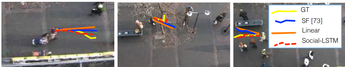
Figure 2.1: Human trajectory prediction in image space; Social LSTM [3] performs predictions on a sequence of RGB images using Recurrent Neural Networks (RNNs).
